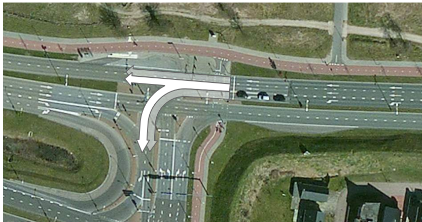
Figure 2-3: Aerial overview of the old situation at the intersection Holterweg–Zweedsestraat in Deventer. The white arrow indicates the switching lane that is now in use.
