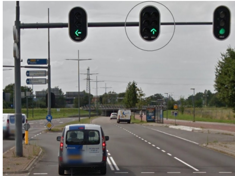
Figure 2-4: Double signal head for the switching lane at the intersection Holterweg–Zweedsestraat in Deventer
